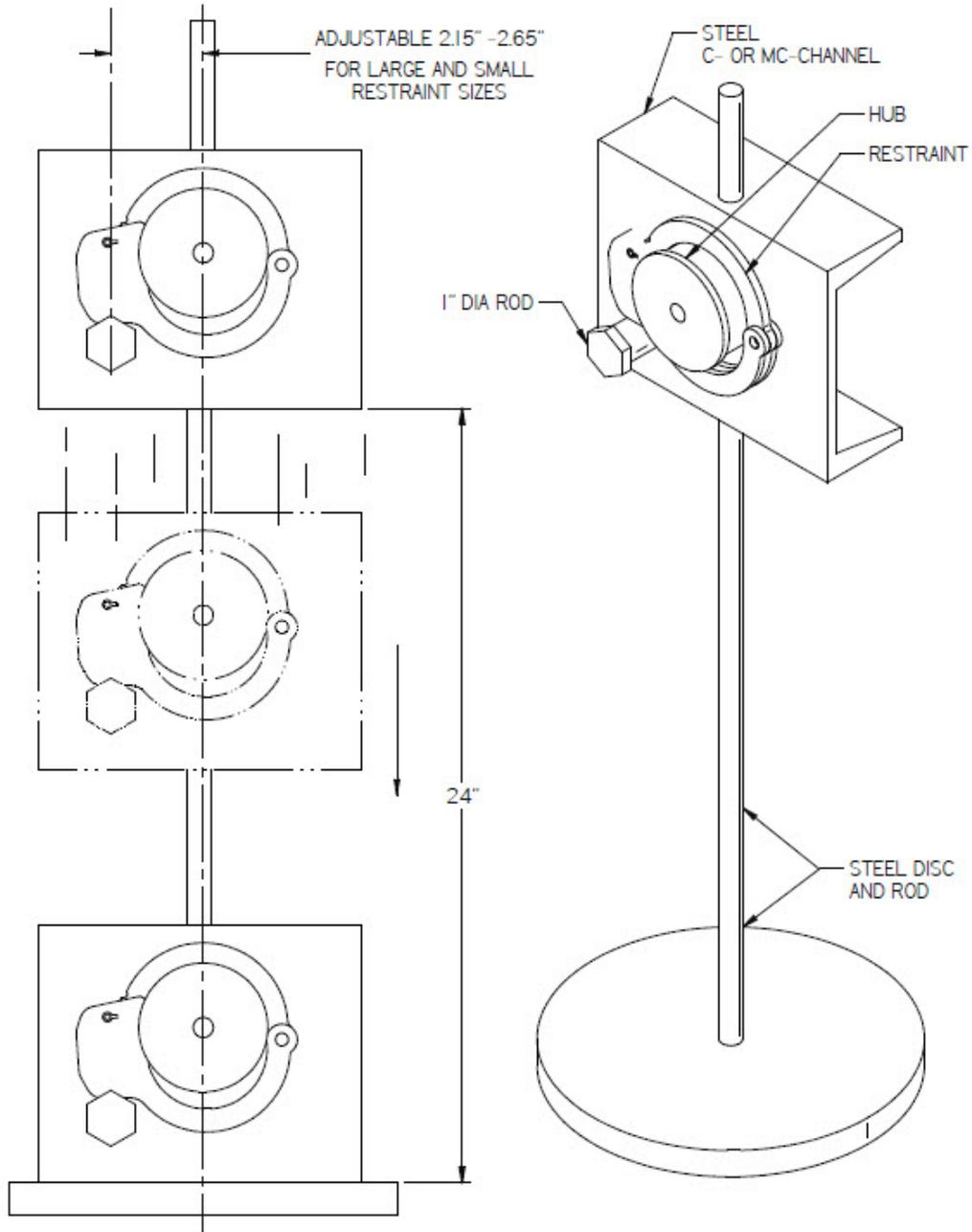
**Figure 17. Compression Test Setup**
