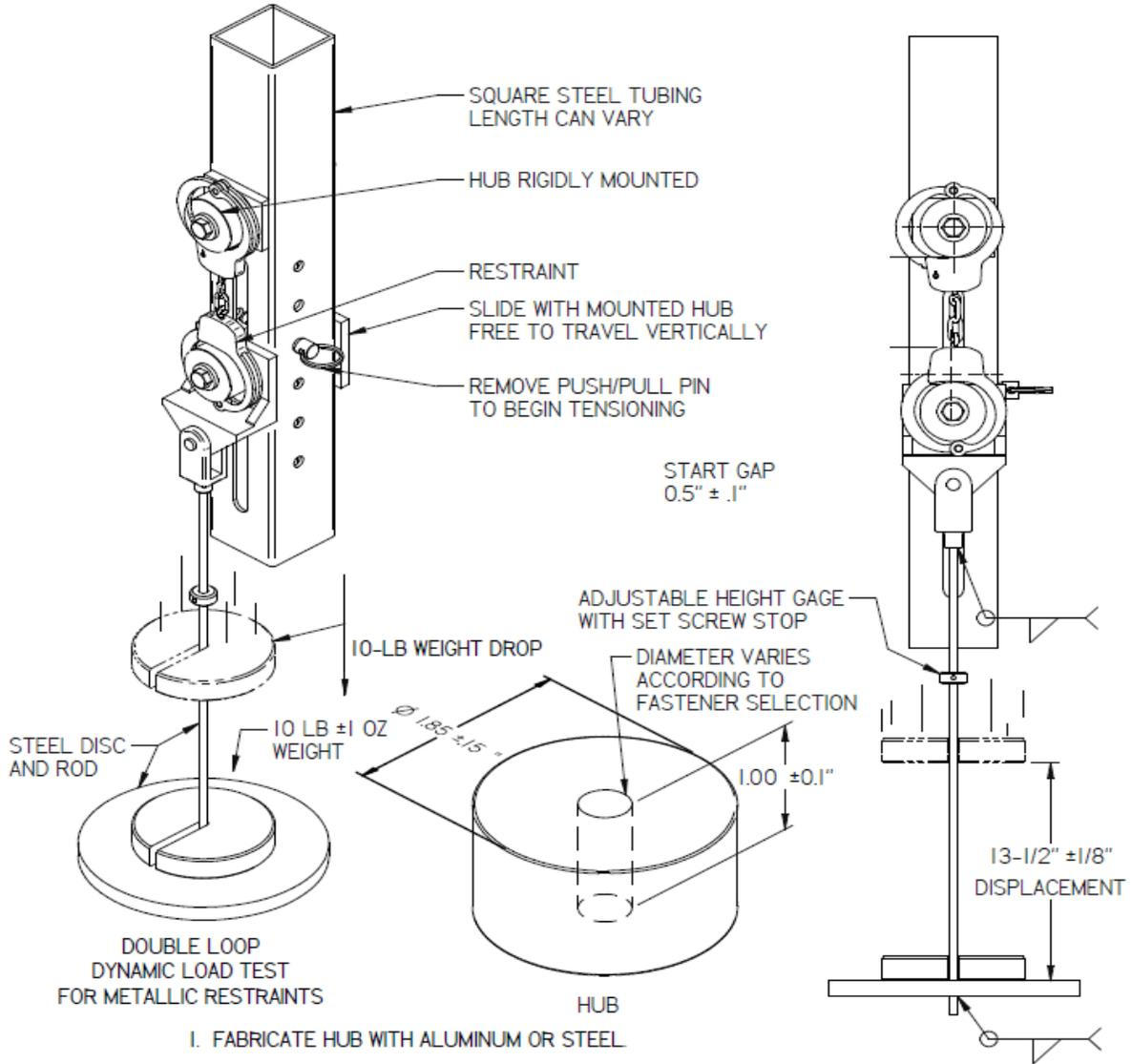
1. FABRICATE HUB WITH ALUMINUM OR STEEL
