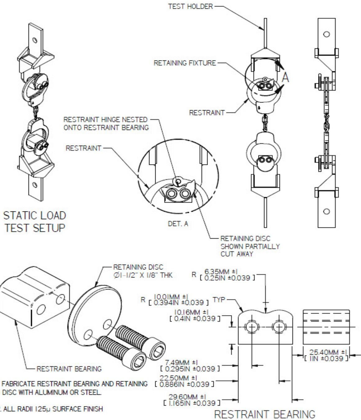
Figure 12. Static Load Test Setup for Individual Loops
