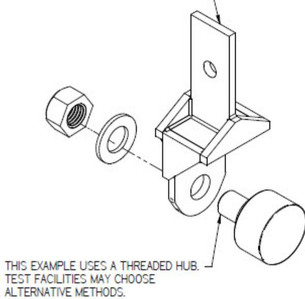
Figure 10. Restraint Retention System Twist Test Setup
