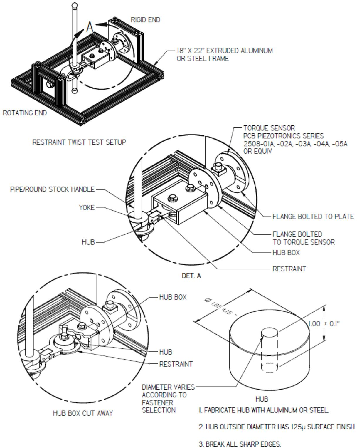
Figure 14. Swivel Pry Test Setup
