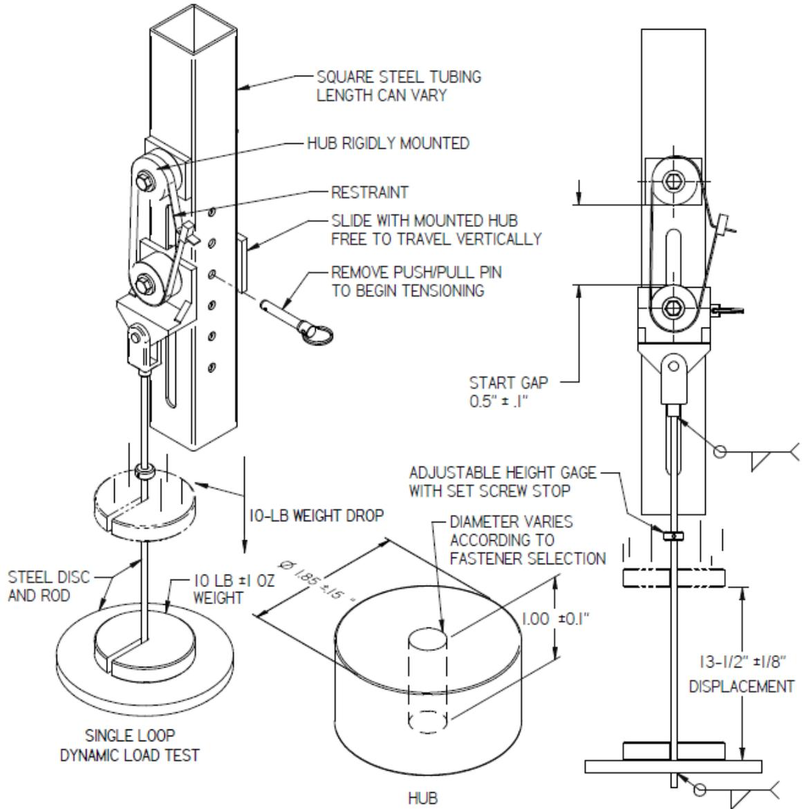
1. FABRICATE HUB WITH ALUMINUM OR STEEL
