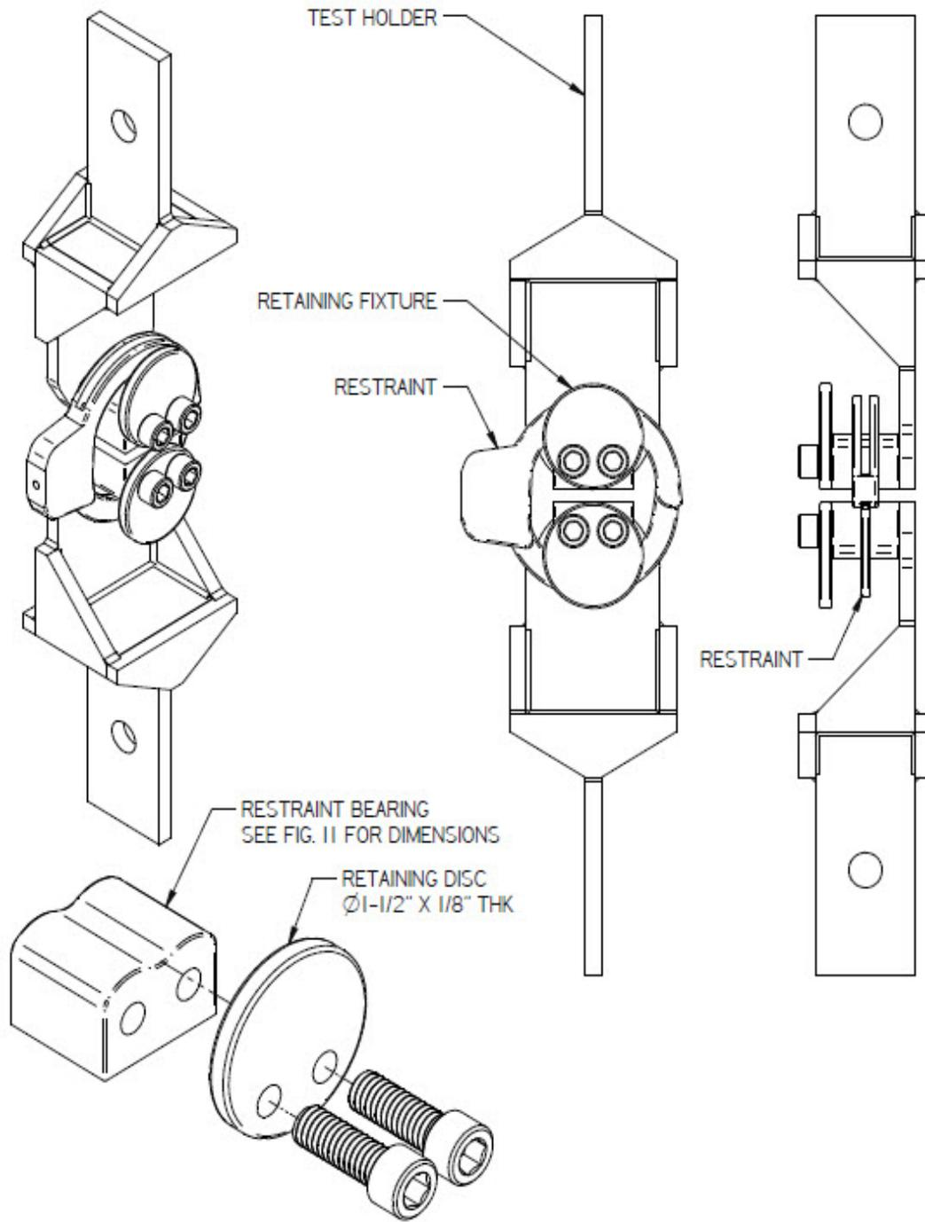
1. FABRICATE RESTRAINT BEARING AND RETAINING DISC WITH ALUMINUM OR STEEL
