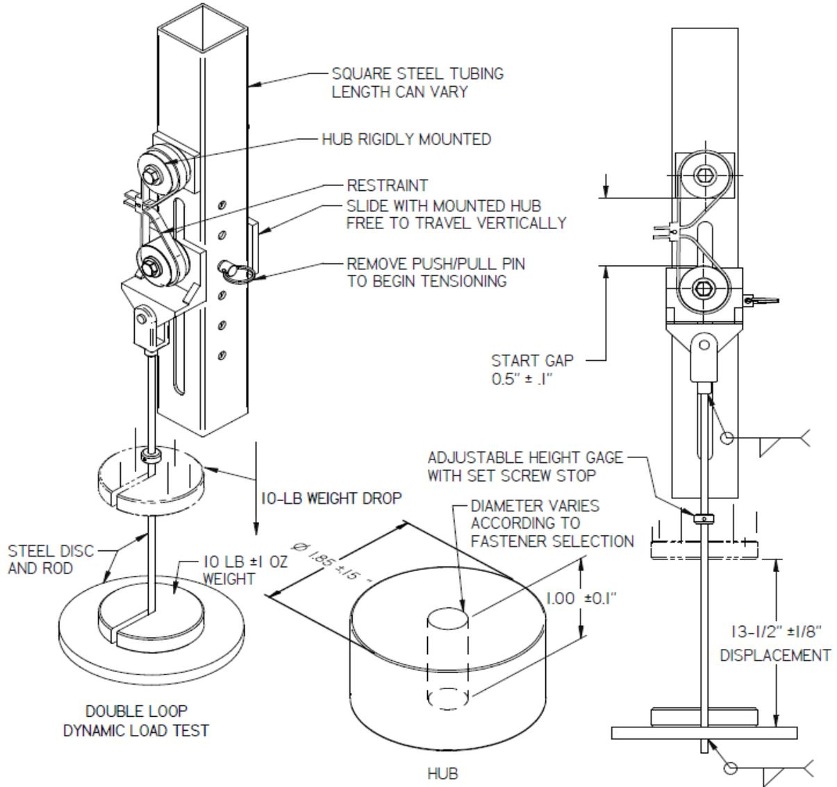
1. FABRICATE HUB WITH ALUMINUM OR STEEL.
