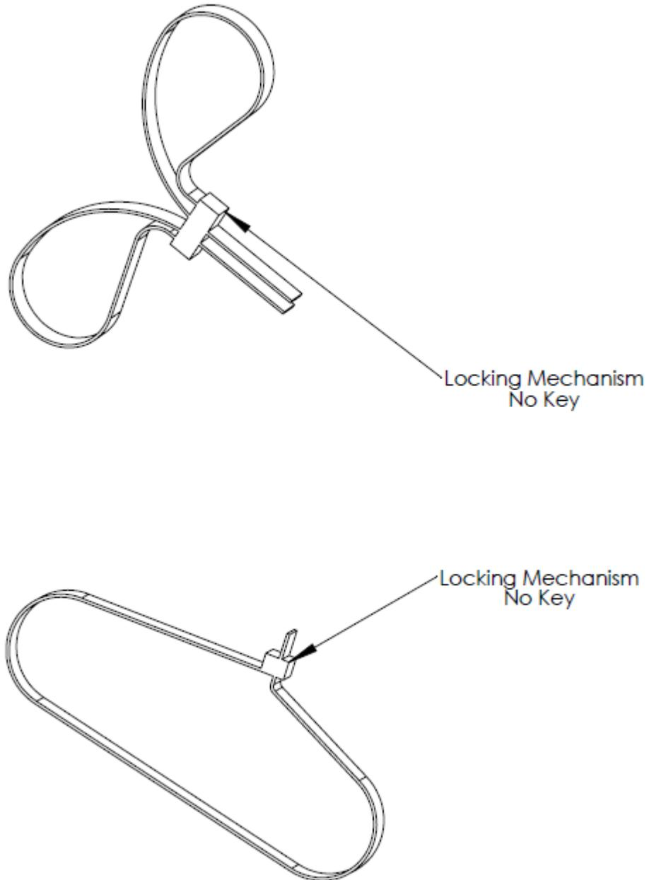
**Figure 2. Examples of Type 2 Restraints**
