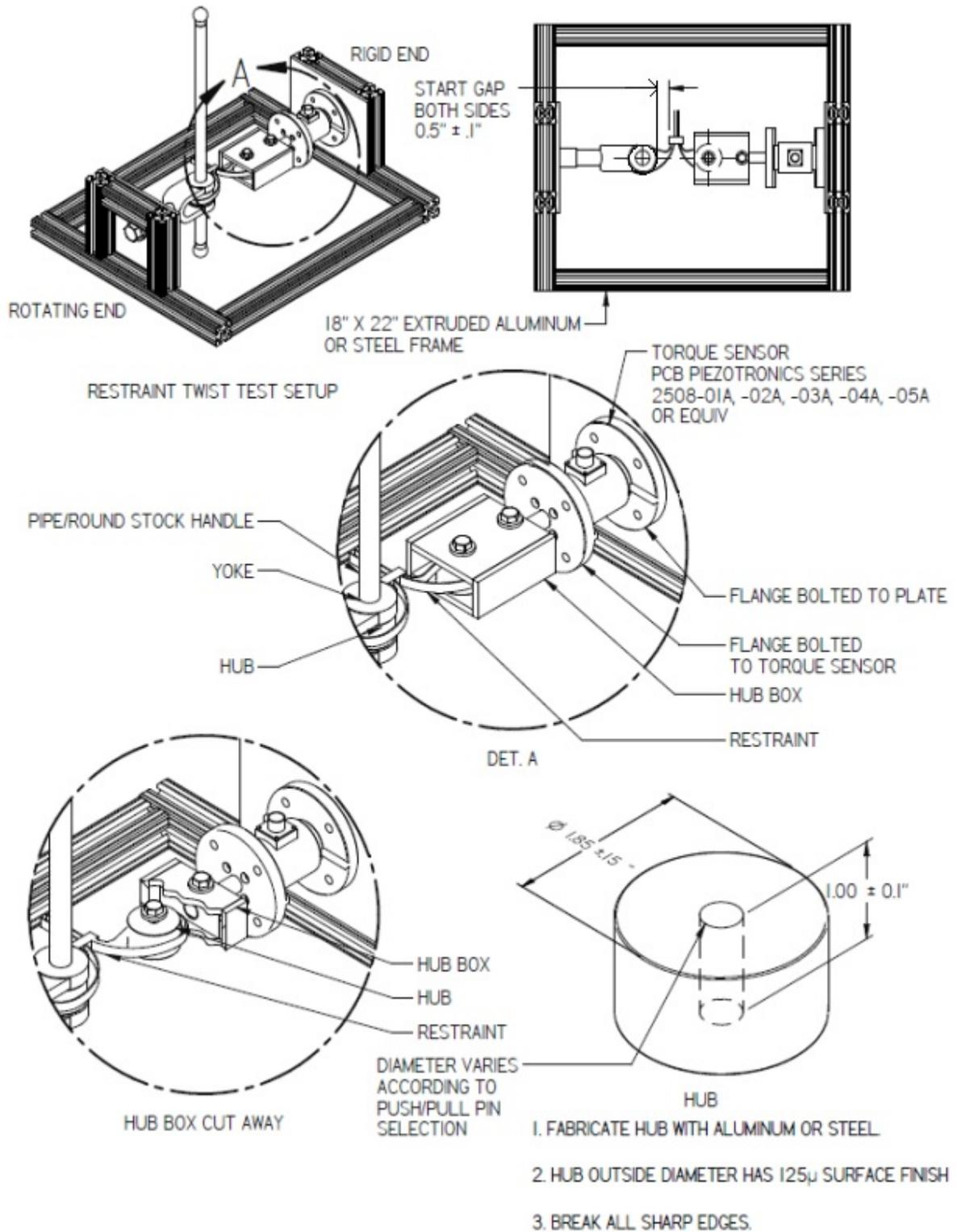
Figure 11. Static Load Test Setup
